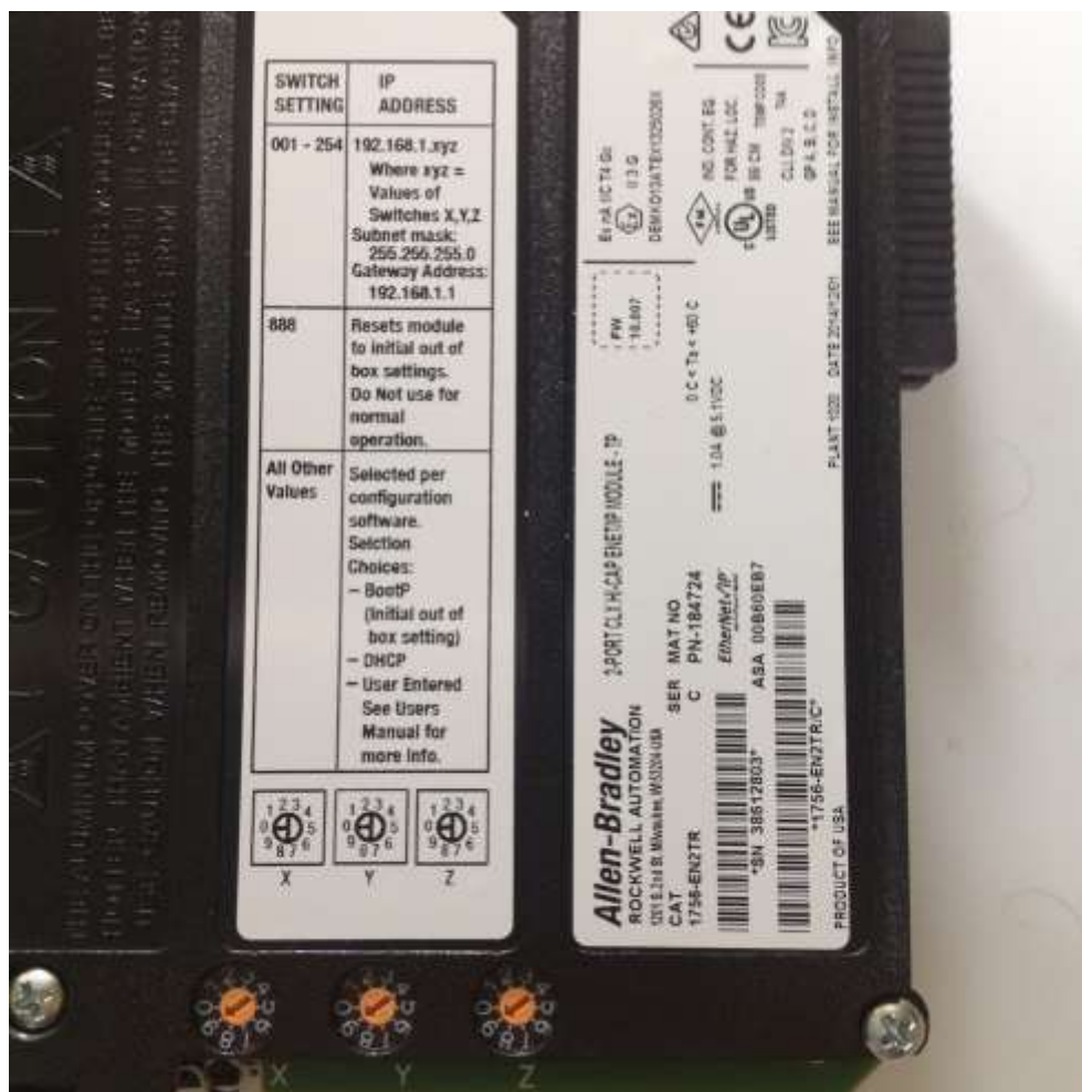
Figure 21-A – Rotary Switches used for manual module configuration
